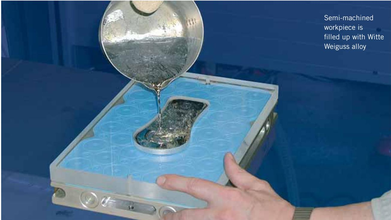
Semi-machined workpiece is filled up with Witte Weiguss alloy
