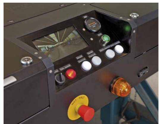
Control panel with camera monitor
