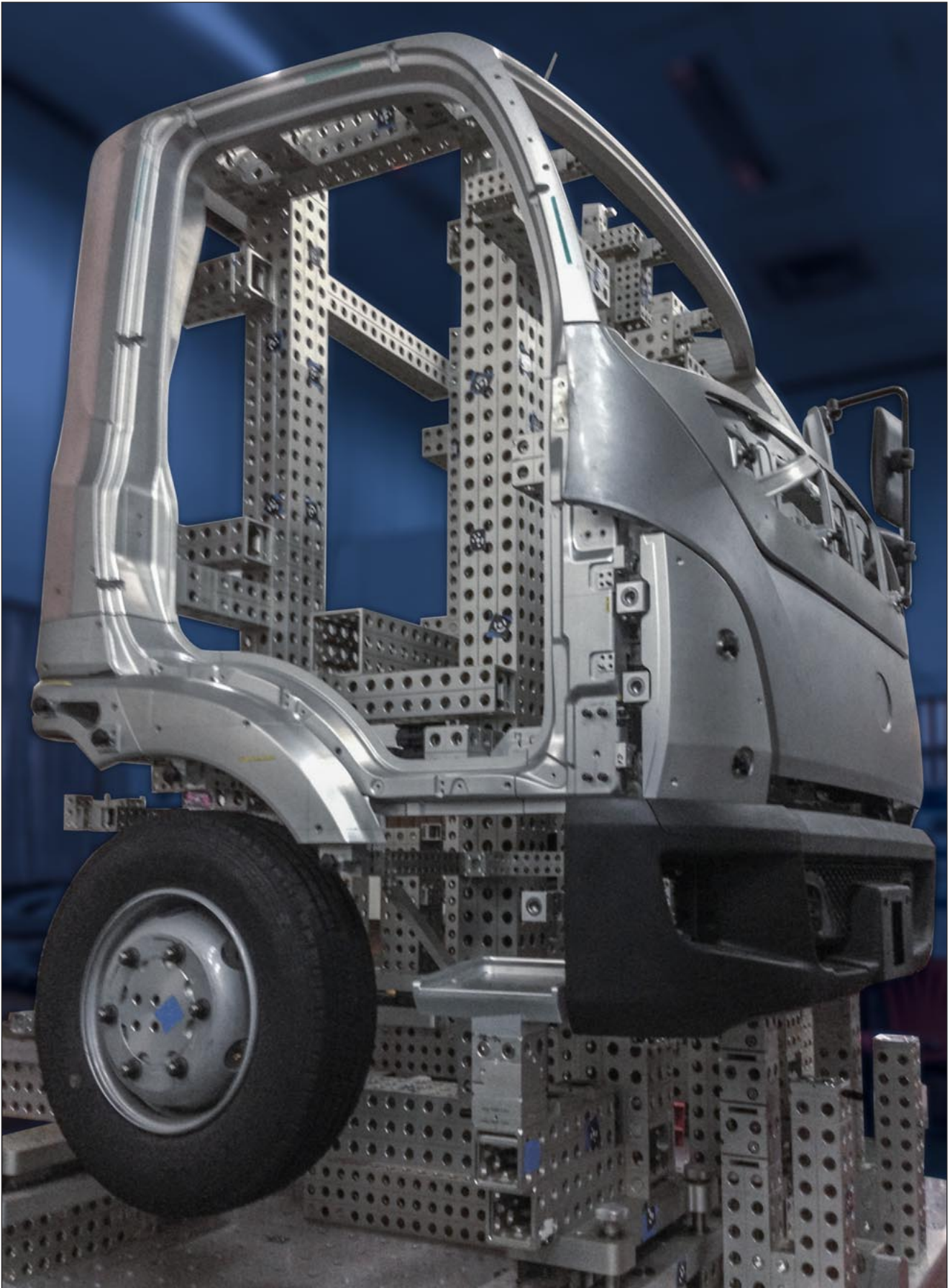
Application example: Fixture for a truck cabin with Alufix Light Classic bars
