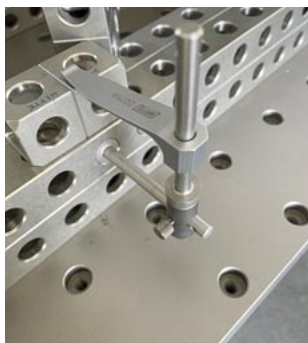
Application example for cross connector with hold down column.
