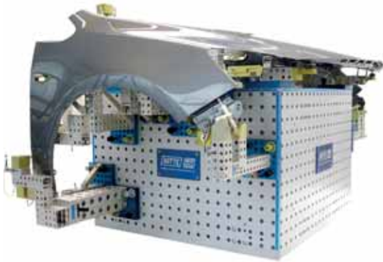
Fixbase Cube for mounting single parts of vehicle front
