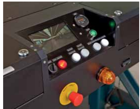
Control panel with camera monitor
