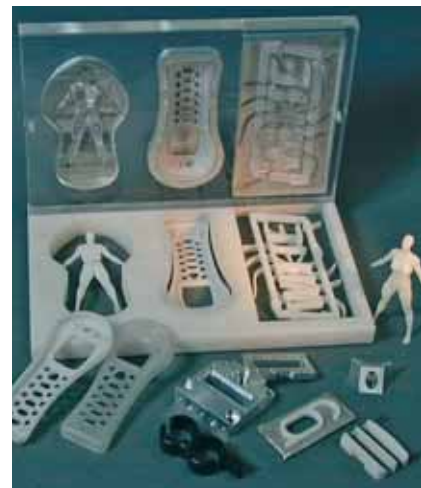
Witte Weiguss is especially suitable for complicated workpieces with curved or concave surfaces
