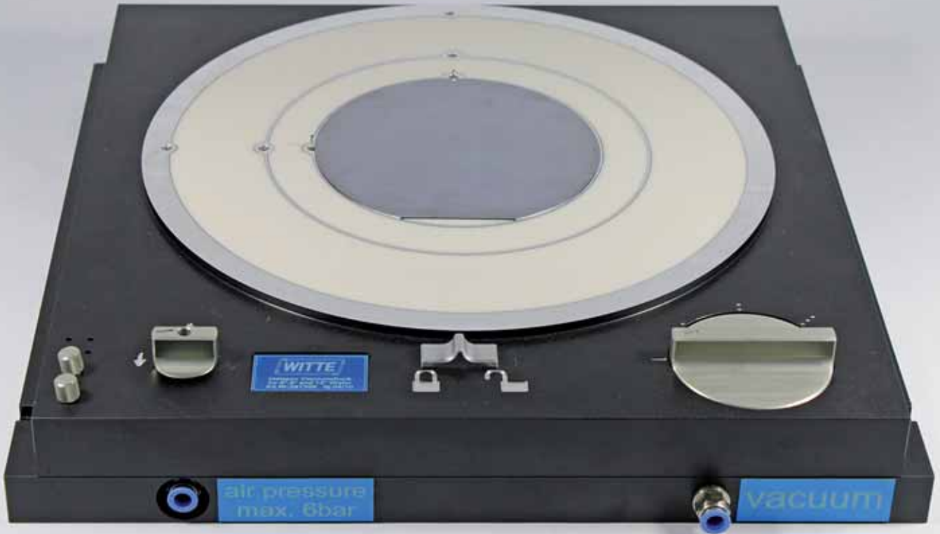
Specially designed porous chuck with three individual clamping areas, stops for part positioning and lifting pins for easy removal of wafers.
