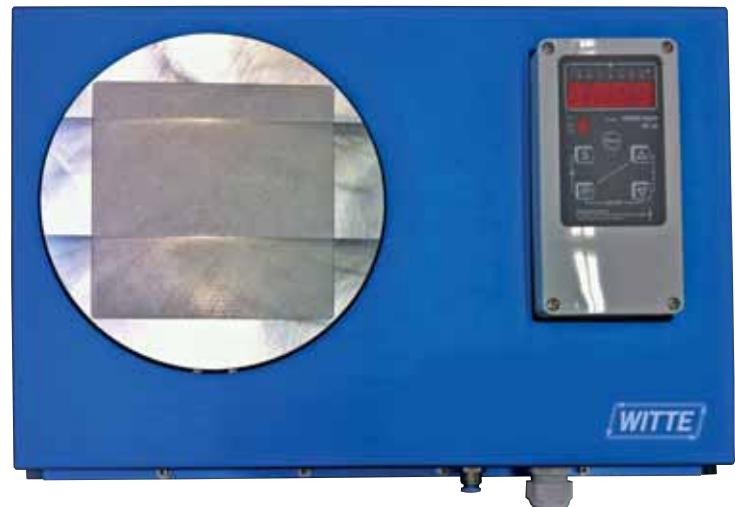
Special version with integrated heating and electronic temperature control
