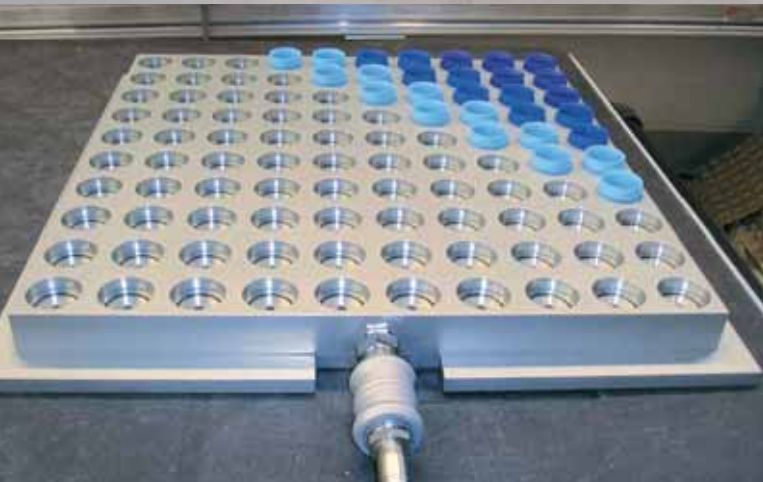
Vacuum chuck for clamping bottles tops during measuring by coordinate measuring machine
