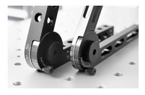
The new angle presetters with vernier scale and positioning in 1-degree steps also promise less complicated, faster and more precise alignment or attachment of workpieces.
