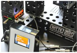
The LEaD positioning aid is offered both as a factory-integrated system in grid plates from Witte and in the form of separate LEaD boxes for fixture assembly with the modular fixturing system ALUFIX from Witte.
